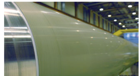
Figure 3. CalJaguar H composite calender roll cover is developed especially for barring-troubled positions.
